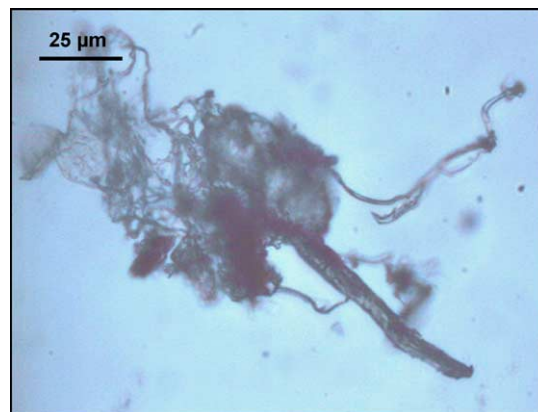
Fig. 8. Microscopic picture of a particle from a freeze-dried suspension from fibre-free MHEC type 10000 B 90%, Elcema® P 050 10%.
